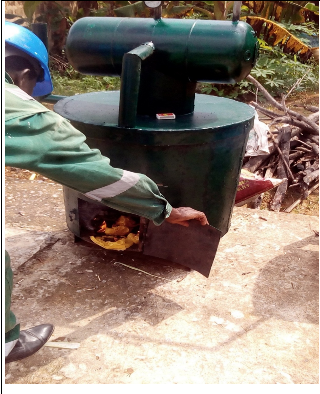
Plate 4.8 Setting fire on the waste in the incinerator
