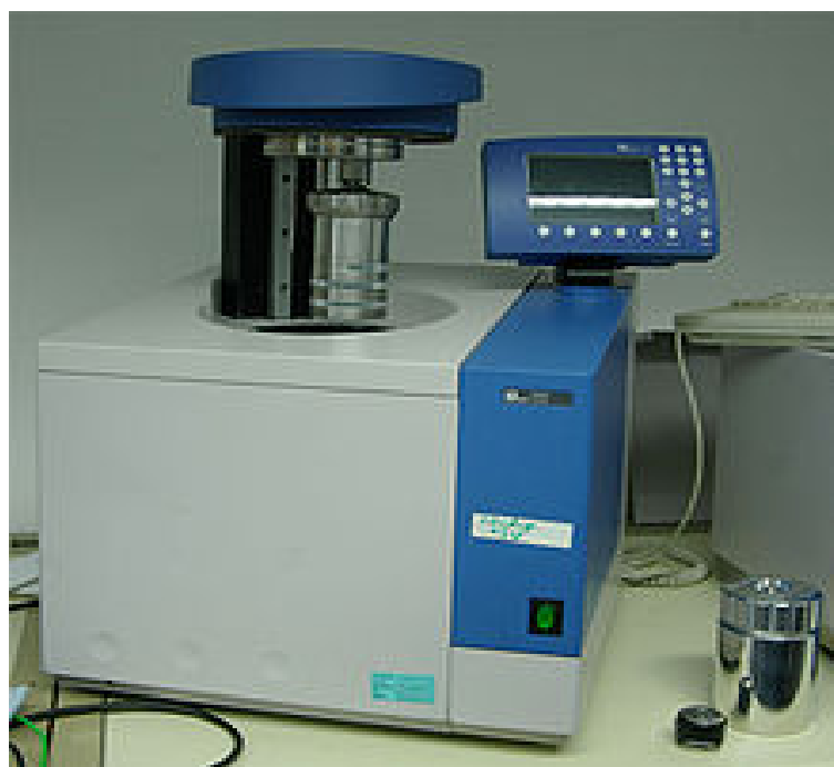
Plate.3.2 pictorial view of the Bomb Calorimeter
