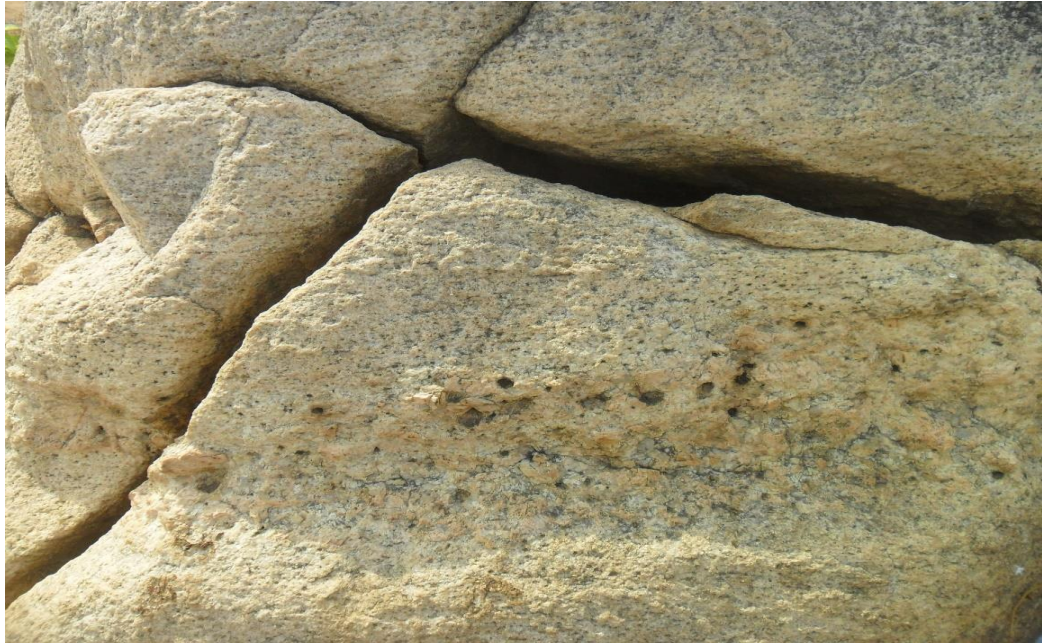
Fig. 4. 32 Open joints in coarse grain granite
