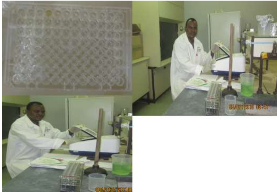
Figure 3.3.3. Micropipette plates and test tubes used for in vitro biological assays and Spectrophotometer being used for taking readings of the reaction products at specified wavelength.
