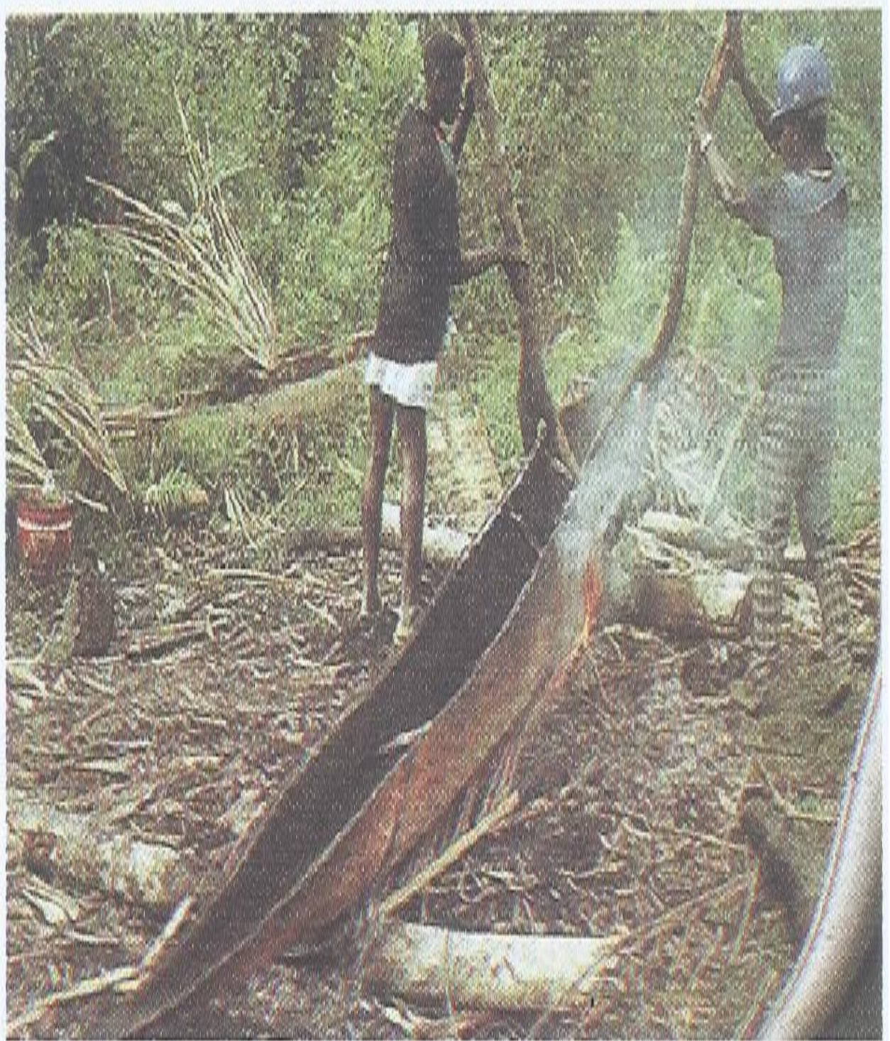
Figure 2.4: A picture showing the process of firing a dug-out canoe, so that it can be bent into shape. Source: Alagoa, E. J. et al. Eds. 2009. The Izon of the Niger Delta... , p. 154.
