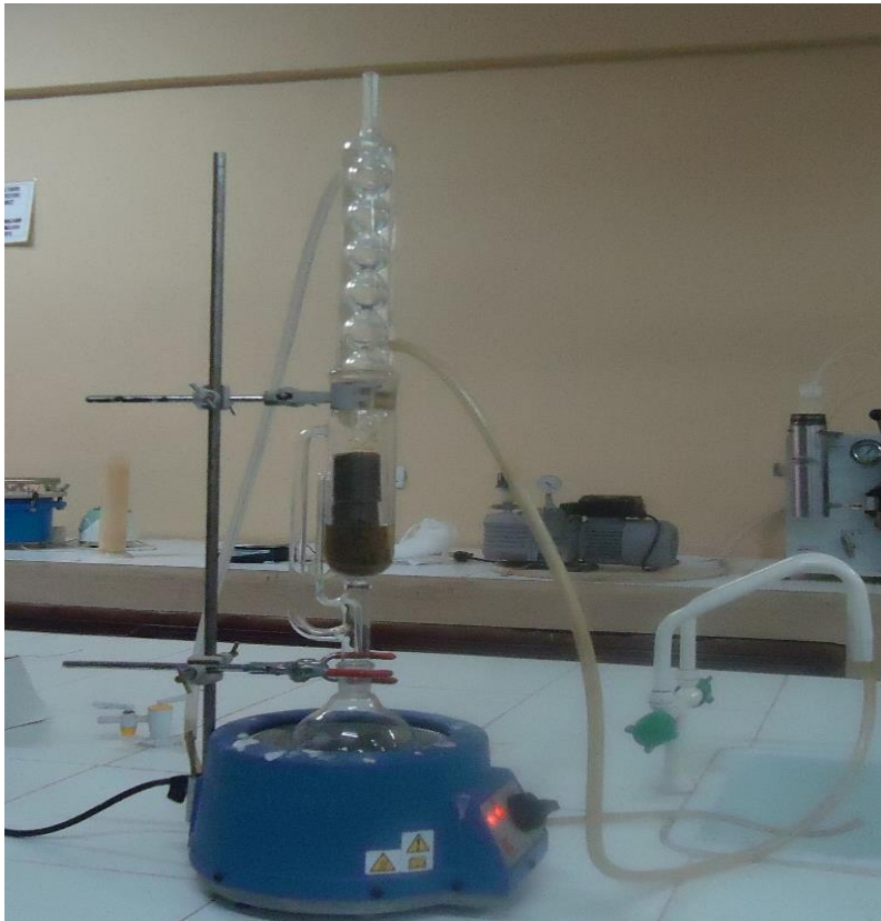
Fig. 3.1: Soxhlet Extraction Apparatus
