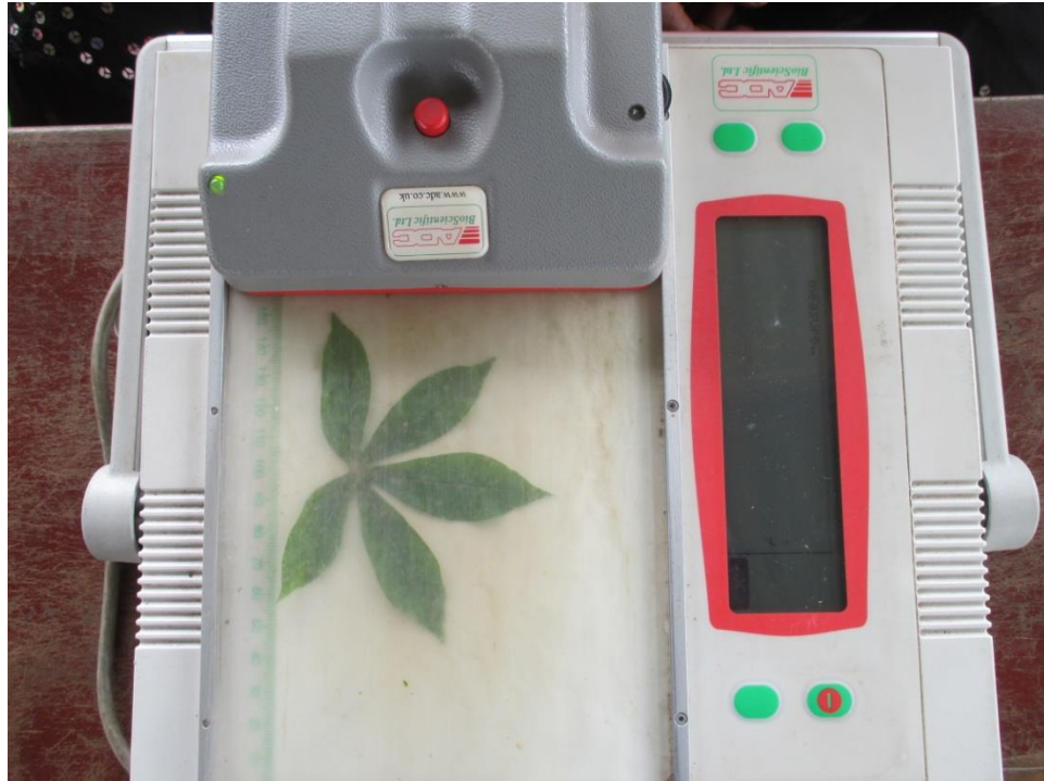
Appendix 17 ADC Bioscience leaf area metre used to measure the length and breadth of cassava leaves in this study
