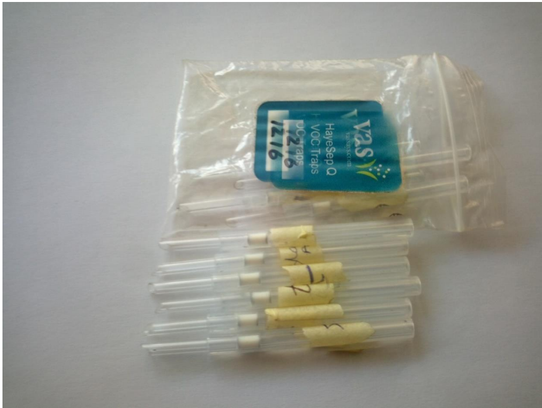
Plate 3.7: Haysep-Q volatile adsorbent trap used for trapping cowpea headspace volatile
