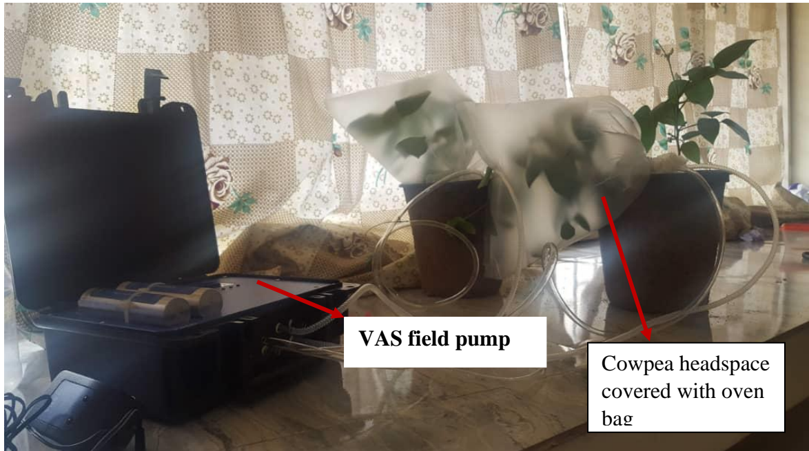
Plate 3.10: The set-up for trapping of cowpea headspace volatiles using the volatile assay systems (VAS) field pump, at the Insect Chemical Ecology Laboratory, Department of Crop Protection and Environmental Biology, University of Ibadan
