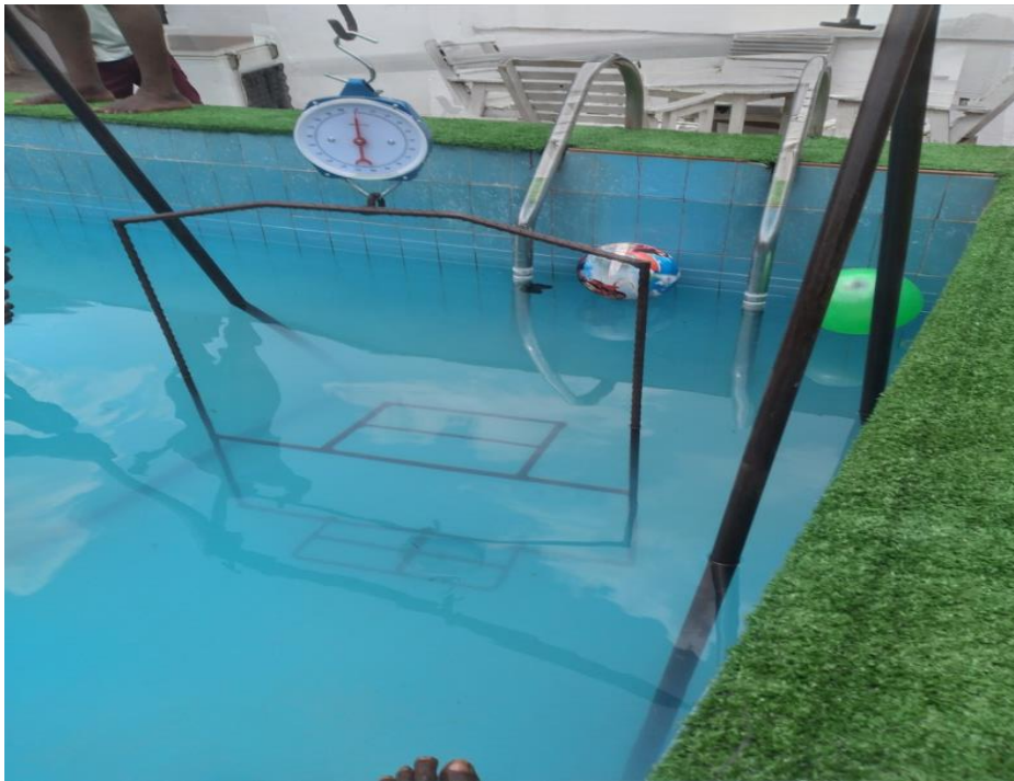
Plate 11; Underwater weighing Equipment inside the pool
