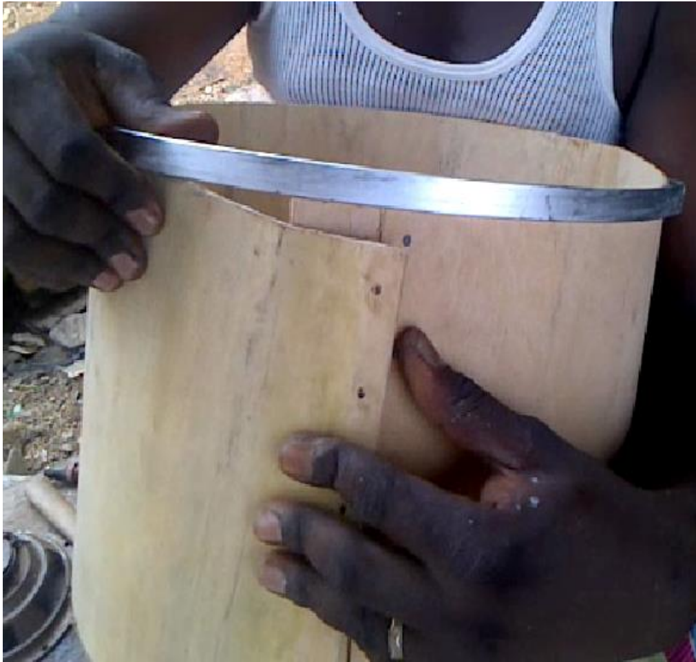
Plate 4.16b: The sheet of plywood is folded to form the round body of the carved wood shape
