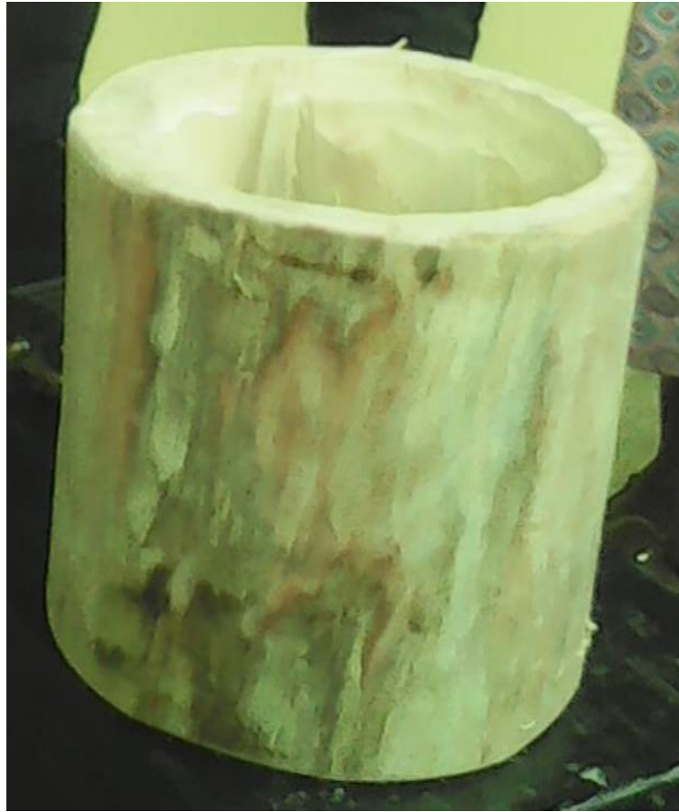
Plate 4.9b): Wooden shell carved from òmò tree log as obtained in bẹ̀mbẹ̀ indigenous technology
