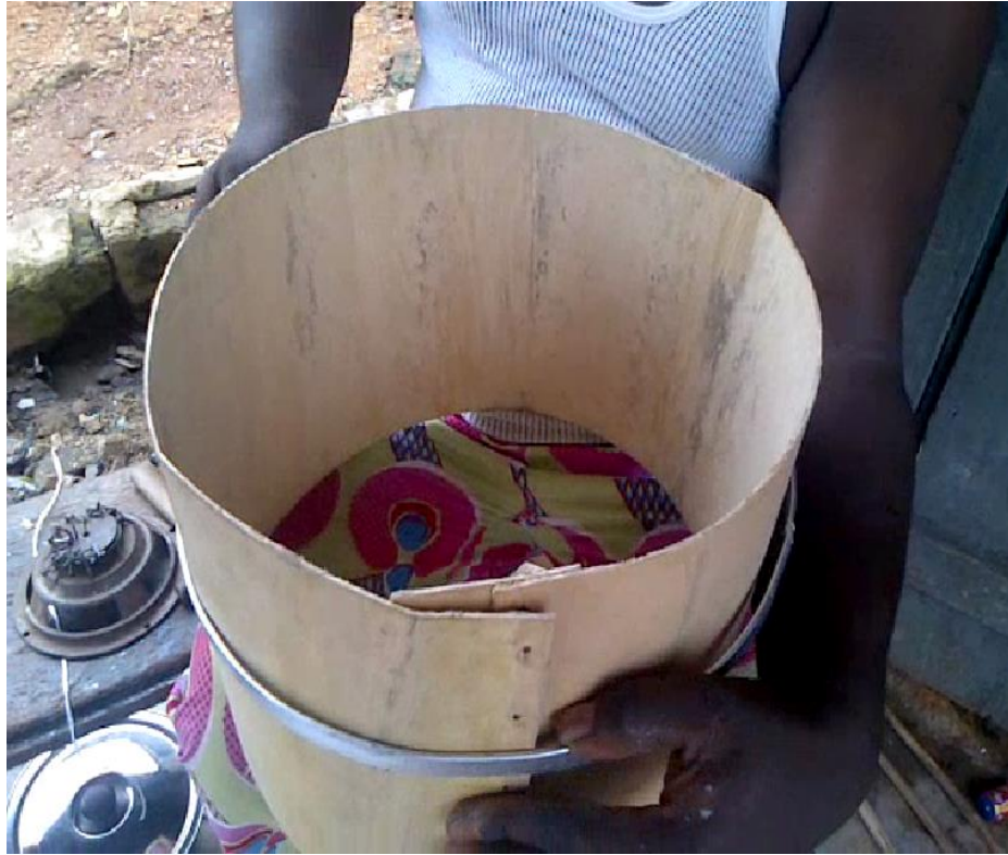
Plate 4.16c The plywood is held to shaped by a round metal bar
