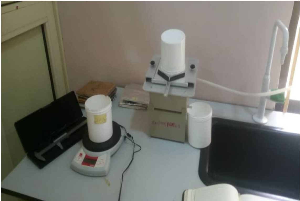
Plate 3.2: Laboratory thermodynamic (ice and steam) apparatus for thermal conductivity
