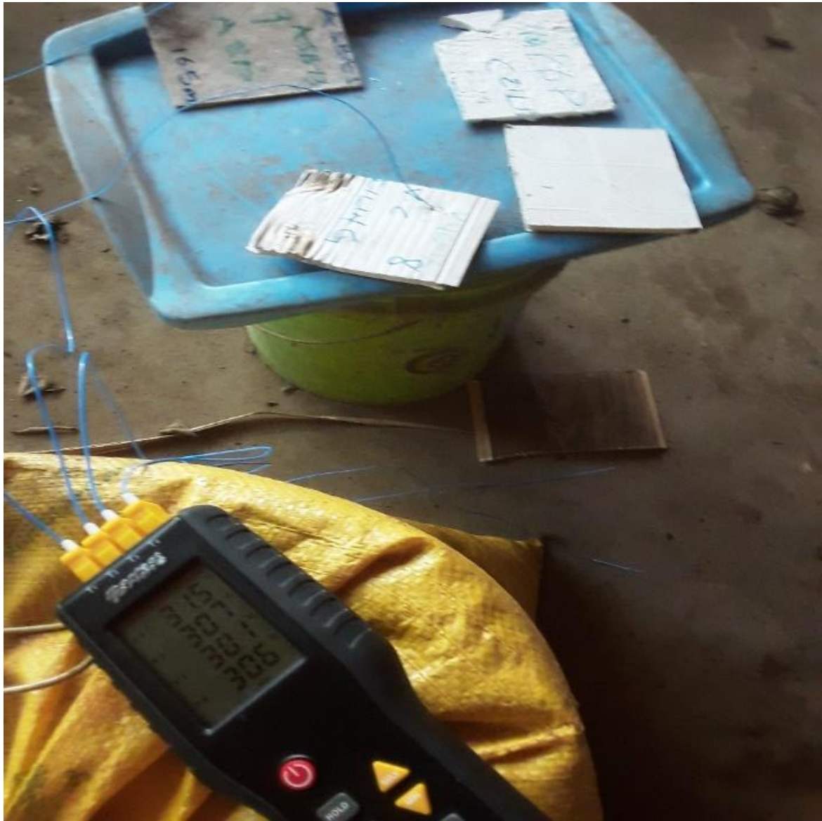
Plate 3.18b: Experimental indoor test for selected ceiling materials
