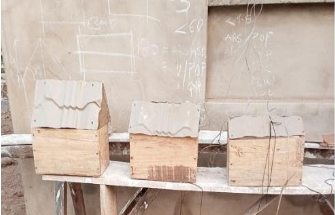
Plate 3.15: Experimental set up for Aluminium roofing sheet with selected ceiling materials
