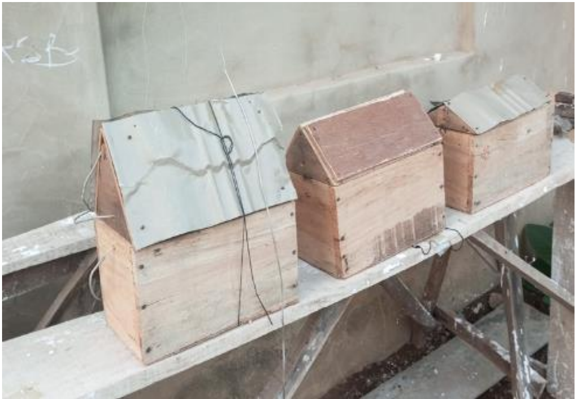
Plate 3.13: Experimental set up for plywood-lined Aluminium roofing sheet with selected ceiling materials
