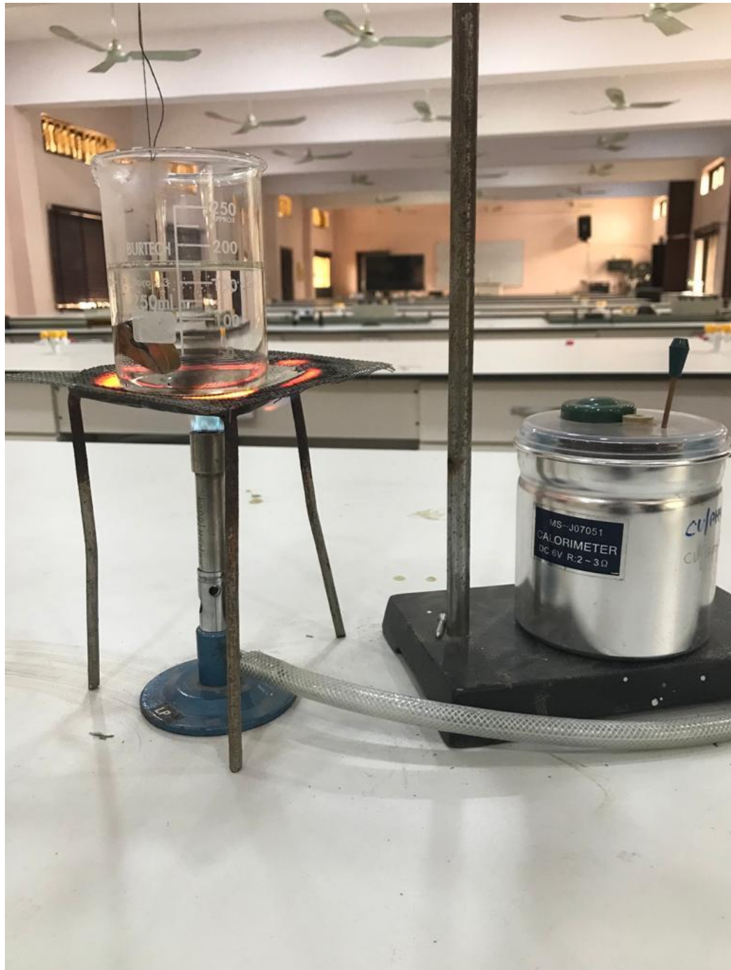
Plate 3.3: Laboratory calorimeter apparatus for specific heat capacity
