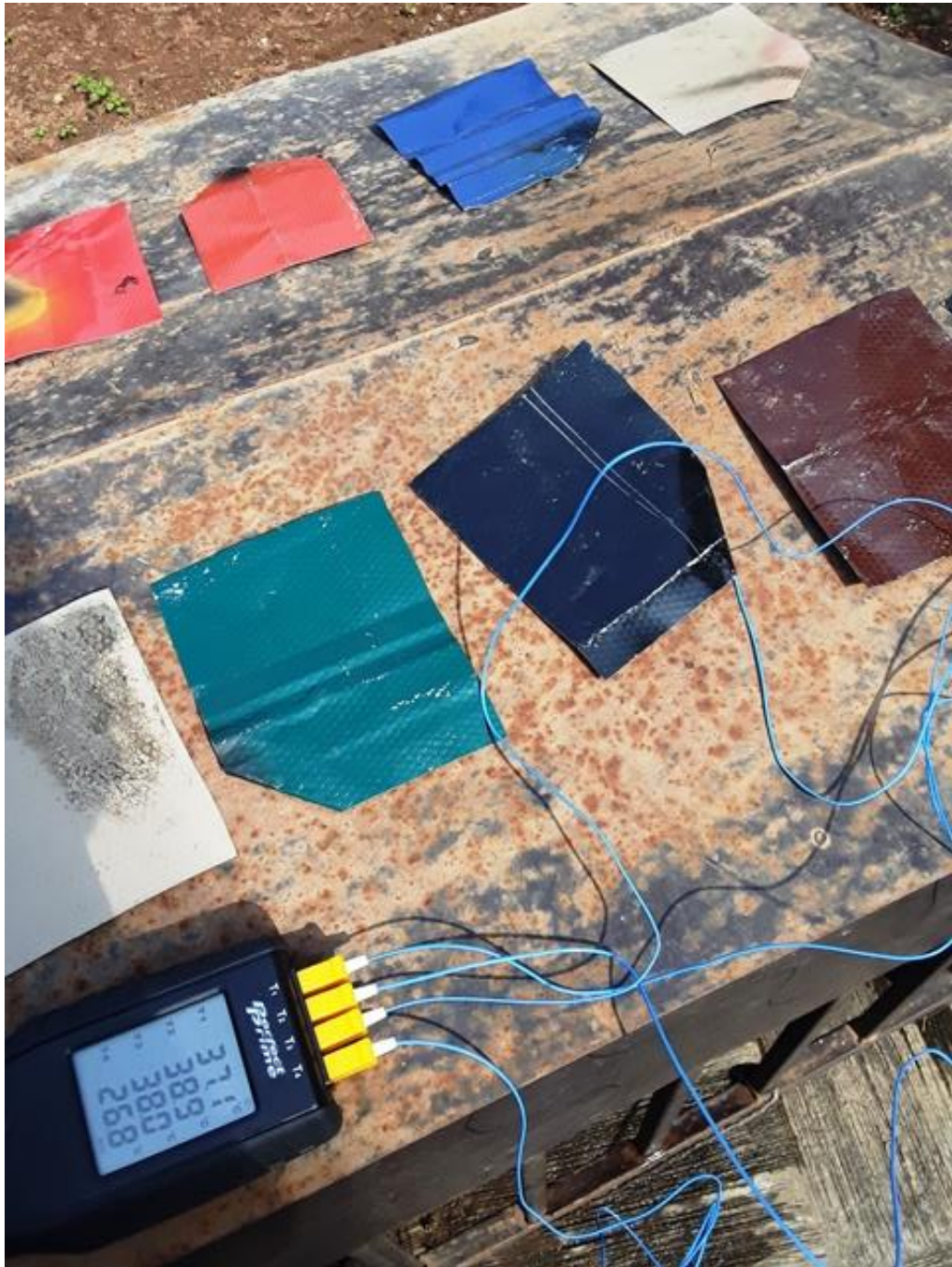
Plate 3.18a: Experimental outdoor test for selected roofing sheets
