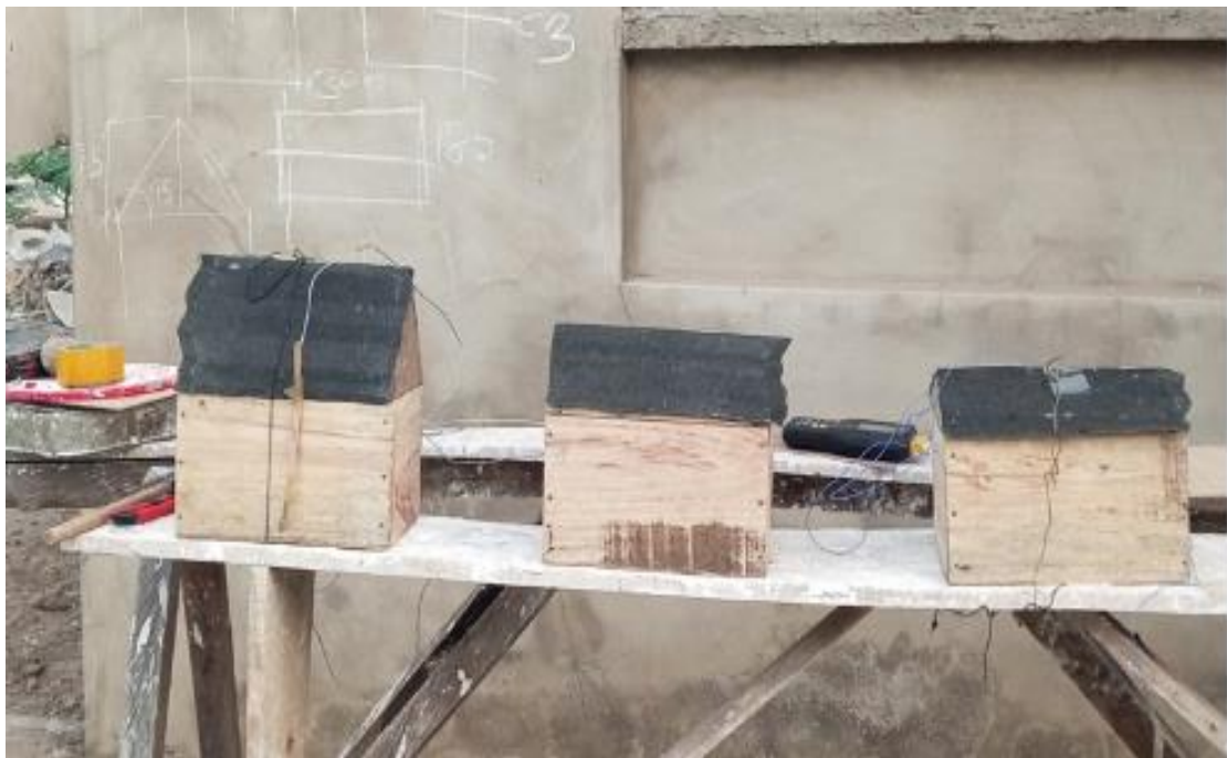
Plate 3.14: Experimental set up for stone coated roofing sheet with selected ceiling materials
