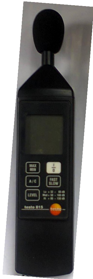
Plate 3.1a: Sound level meter (TESTO 815, Test Equipment Depot, United State of America)
