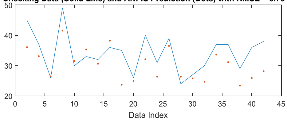
Checking Data (Solid Line) and ANFIS Prediction (Dots) with RMSE = 5.7514
