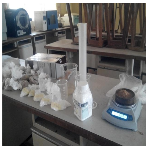
Plate 3.2(a): Pulverized Sieved Precursor Plate 3.2(b): Weighing Balance and Activation Process
