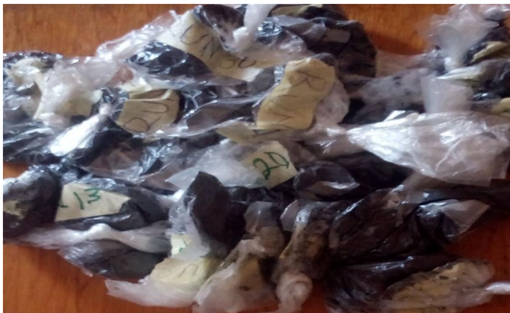
Plate 3.2(c): Phosphoric Acid-modified and Carbonized RPSAC in Preservation Bags
