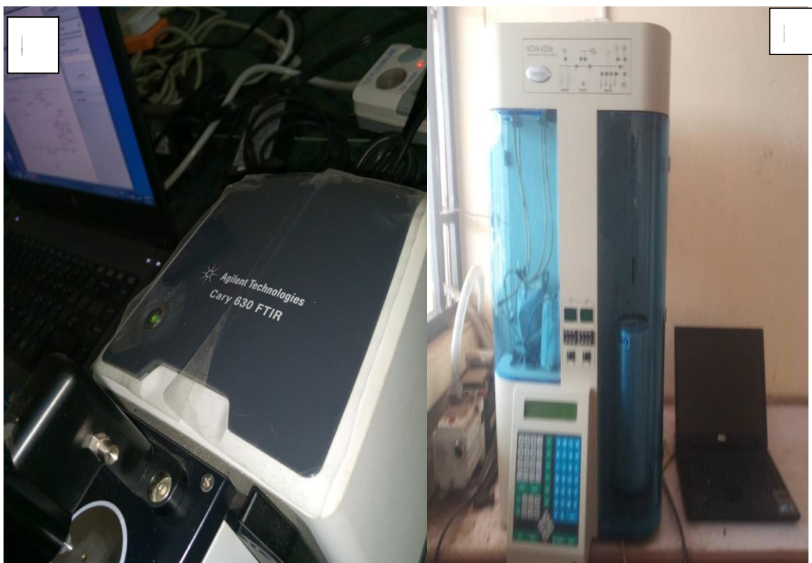
Plate 3.4, (A): FTIR Instrumental Set-up, (B): BET Surface Area and Porosity Analyser
