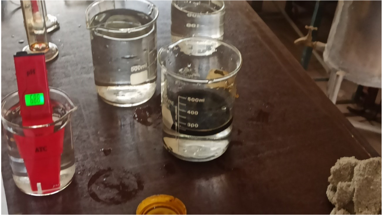
Plate 4.9: Simulated Oil Spilled water and Calibration of pH meter
