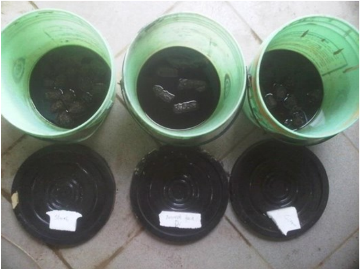
Plate 2.4: Starch, Animal Feed and Cissus bonded Kenaf Pellets During Oil Absorption Test ( Source: Kadiri, 2014 )
