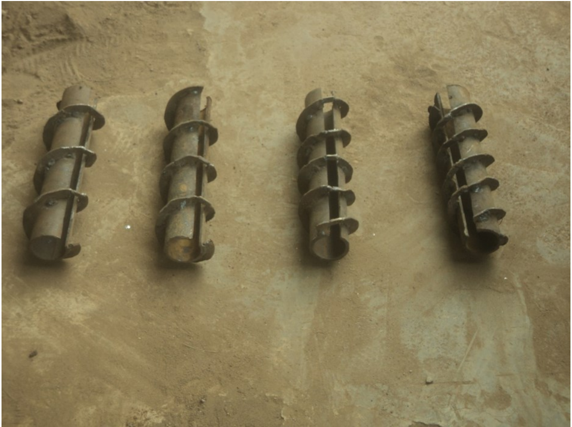
Plate 4.2: Augers used in the Pelletizer.
