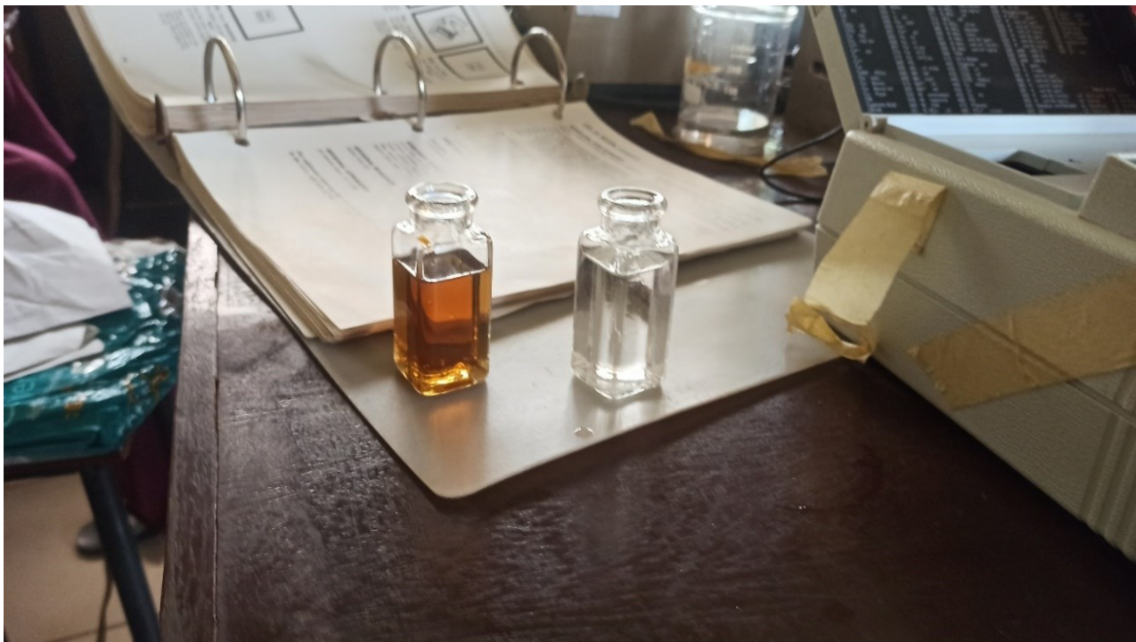
Plate 4.11: Oil Precipitate in Reagent and Blank Reagent Samples
