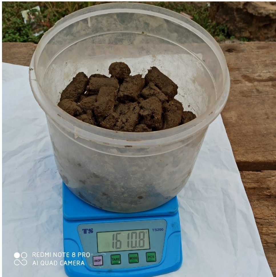
Plate 4.4: Weighing of Freshly Produced Kenaf Pellets
