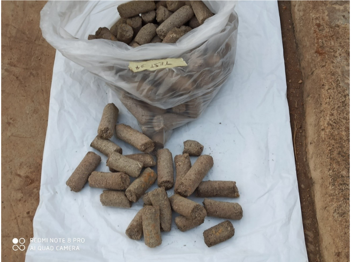
Plate 4.6: Kenaf Pellets Ready for Storage
