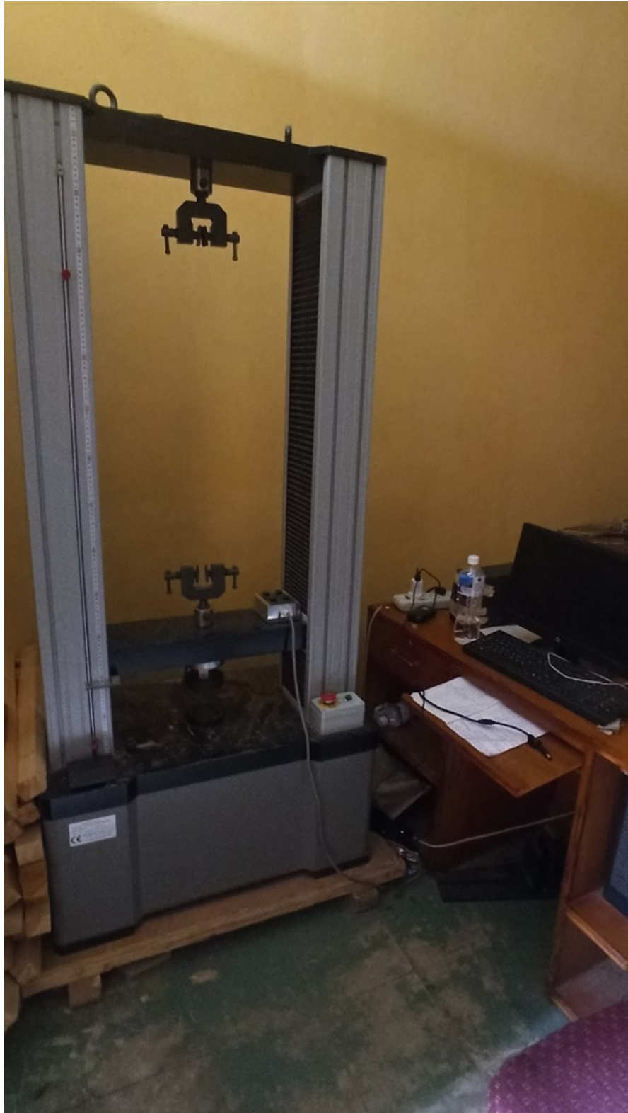
Plate 4.6: Computer Controlled Universal Testing Machine
