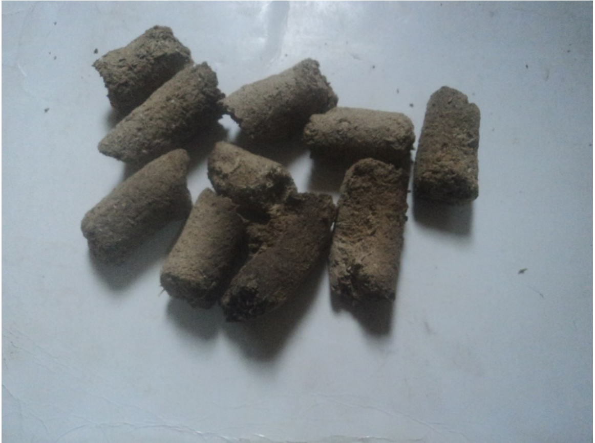
Plate 4.7: Dried Starch bonded Kenaf pellets
