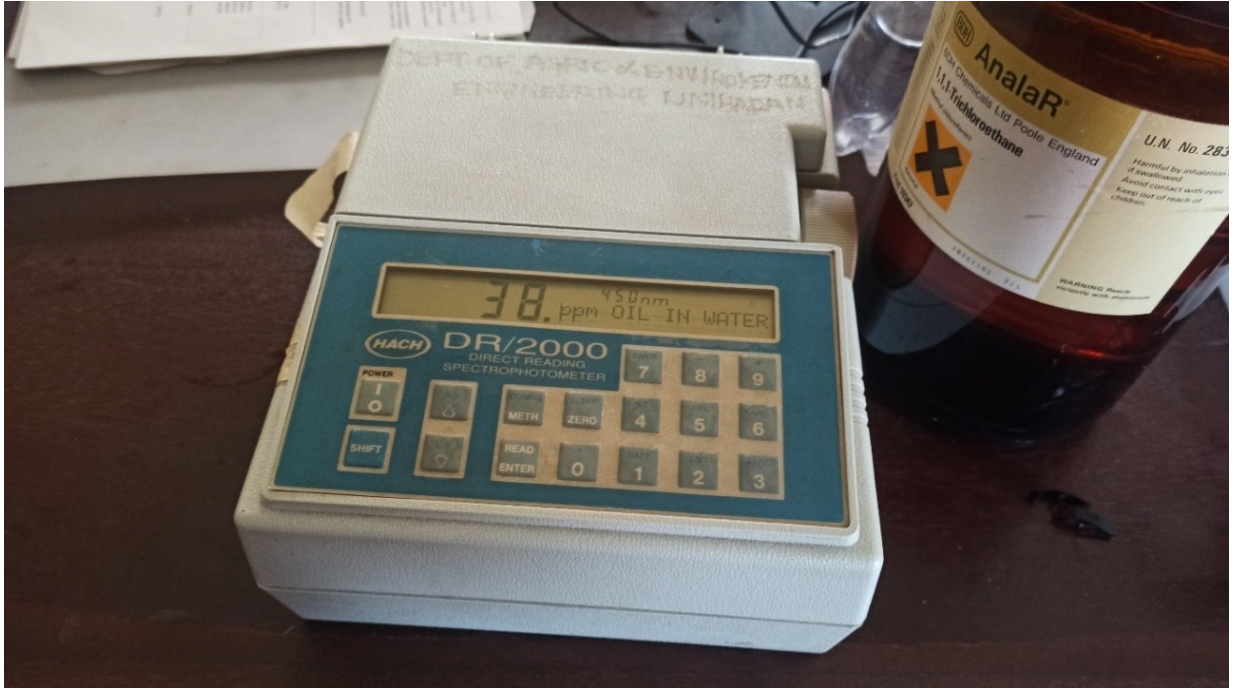
Plate 4.12: Reading of Oil in Water PPM after Remediation.
