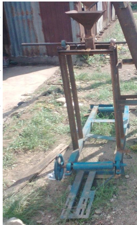
Figure 3.13: (A) Design drawing of metering device and Belt Conveyor (B) Design drawing of Roller and belt (C) Picture of the constructed metering device and belt conveyor
