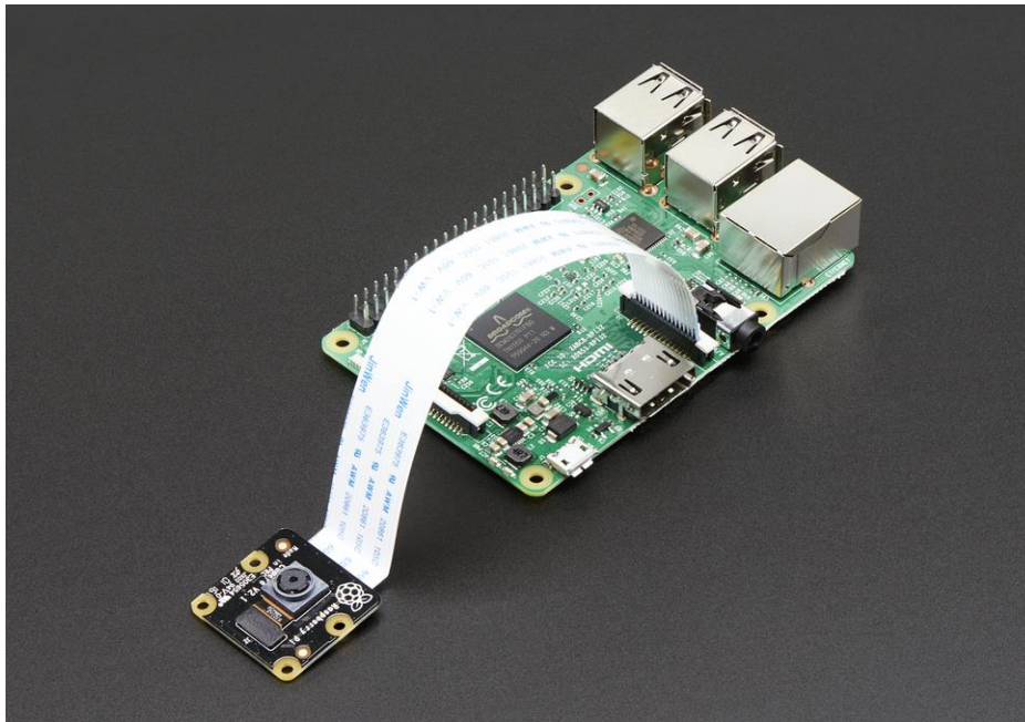
(b) Raspberry Pi NoIR camera board connected to Raspberry pi 3 board
