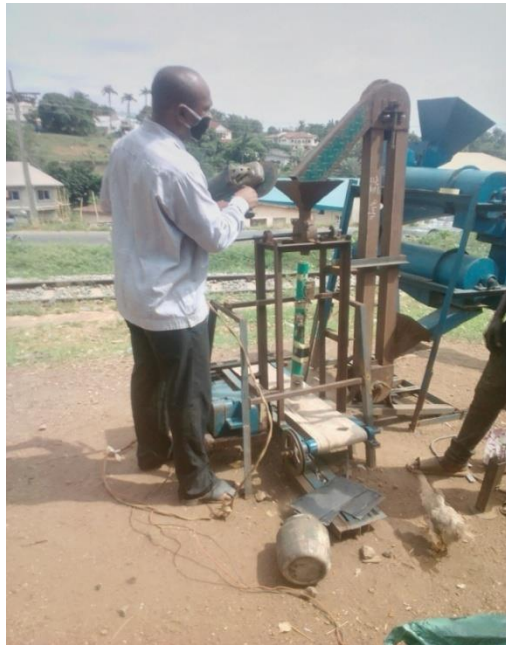
(c) Assembling of bucket conveyor units
