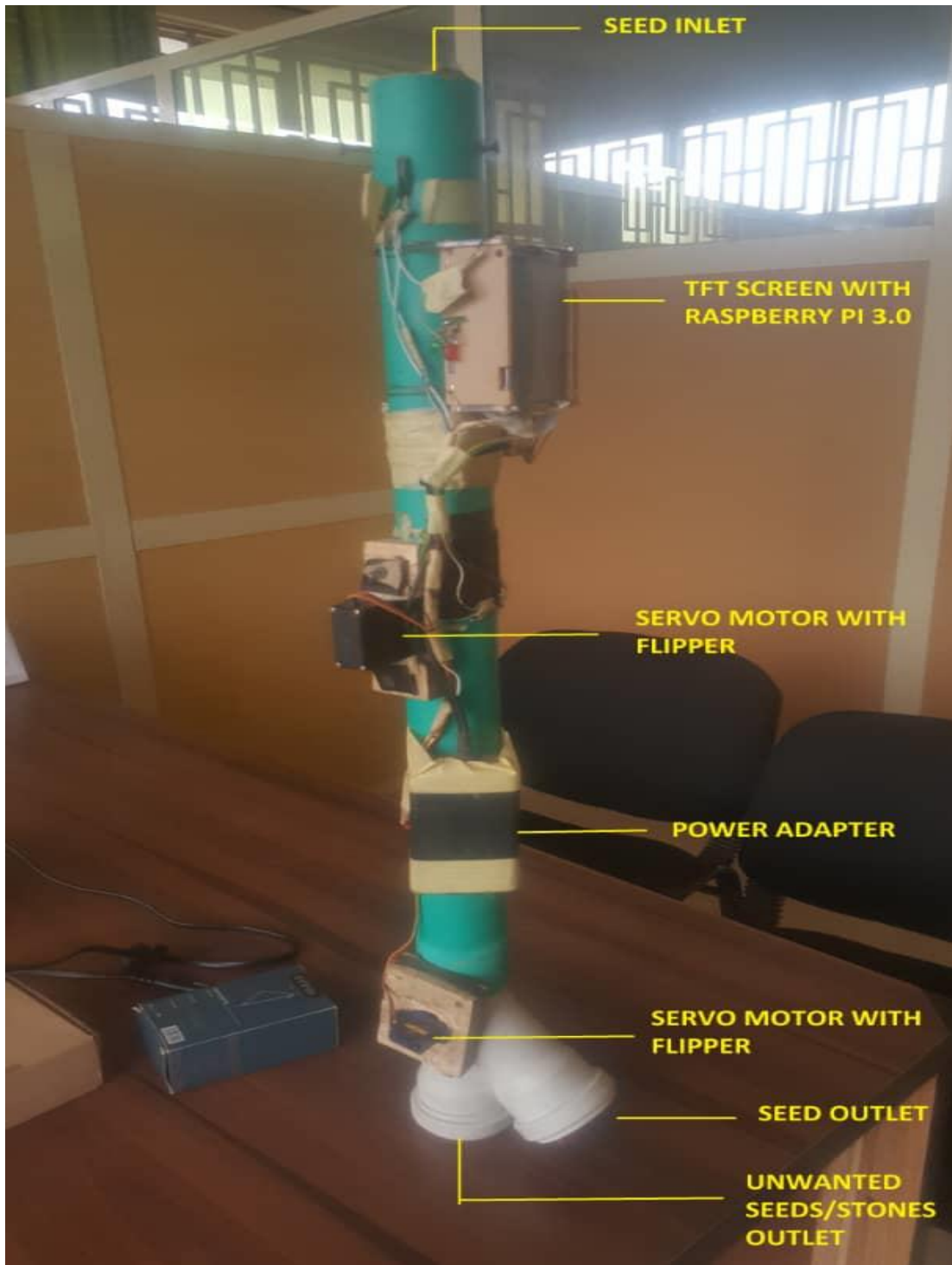
Plate 3.3: Assembled components of the automation units
