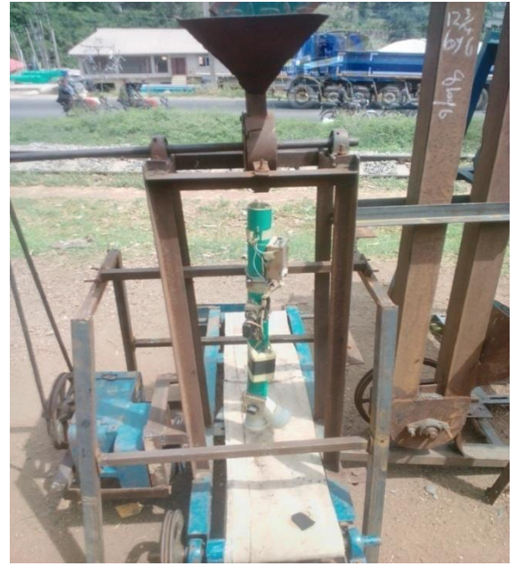
(b) Assembling metering and automation units
