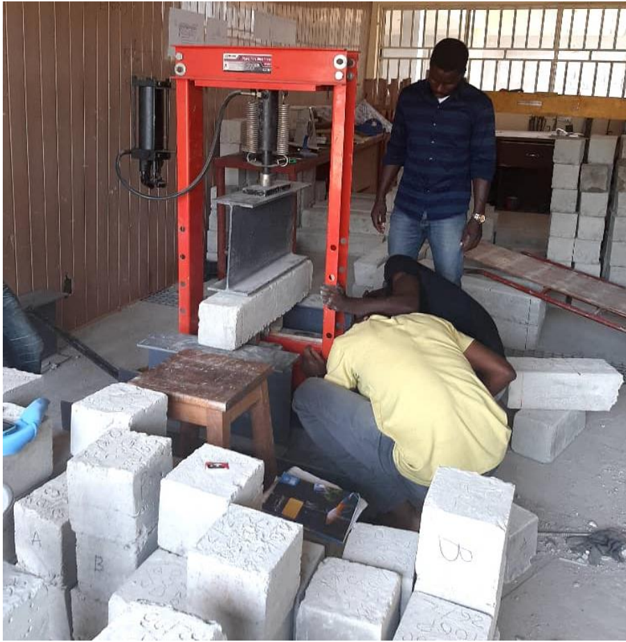
Plate 3.1: Flexural strength testing of cement blended concrete beams
