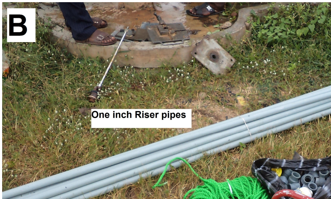
Plates 3.1: Equipment for the conduct of Pumping and Recovery tests at Ibarapa
