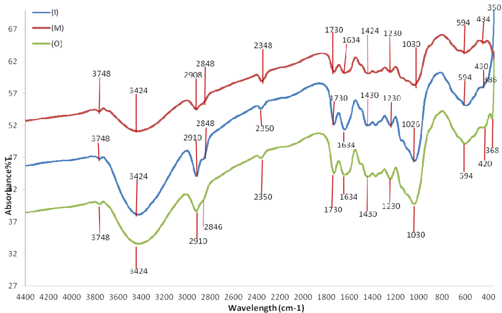
Figure 4.8: FTIR spectra of 20years top wood of tapped Hevea brasiliensis collected from Agbarha rubber plantation, Delta State, Nigeria
