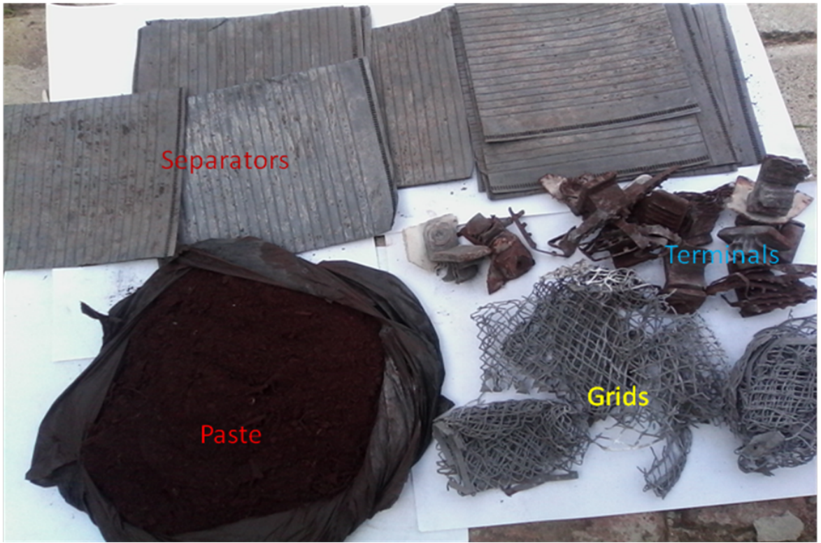
Plate 3.3: Material components of waste lead acid battery (LAB)
