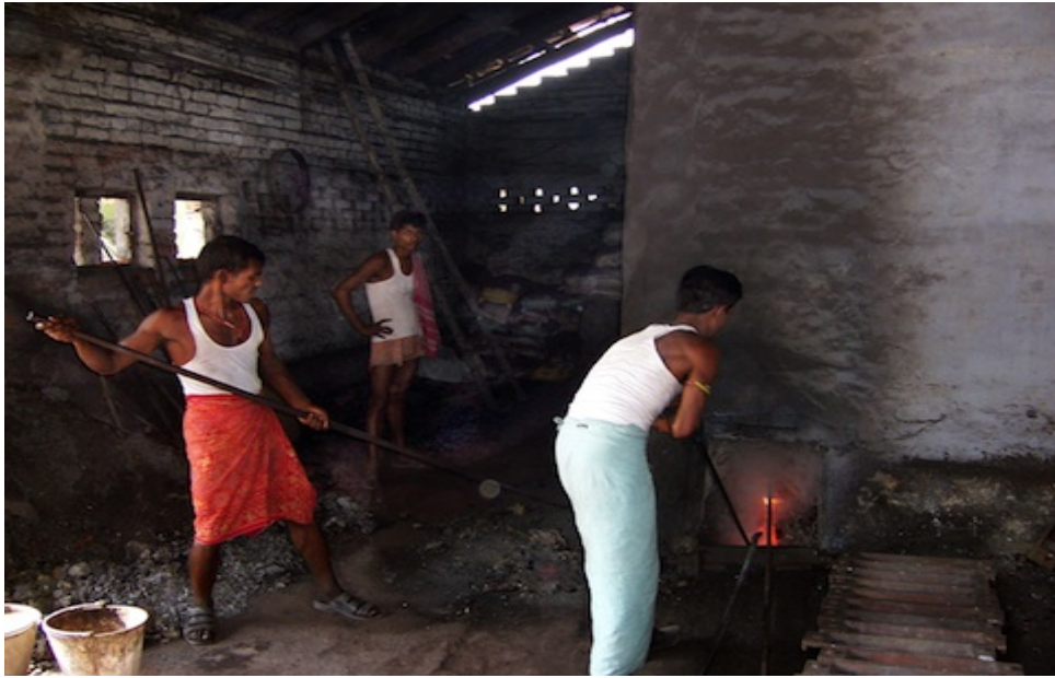
Plate 2.1: Crude smelting of used lead acid batteries
