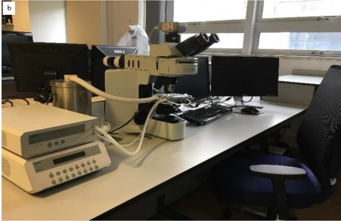
Figure 3.3: Transmitted Plane Polarised Light Microscope fitted with a stage mounted Linkam heating and cooling stage used for microthermometric analysis of fluid inclusions at Geofluids Research Laboratory, National University of Ireland, Galway
