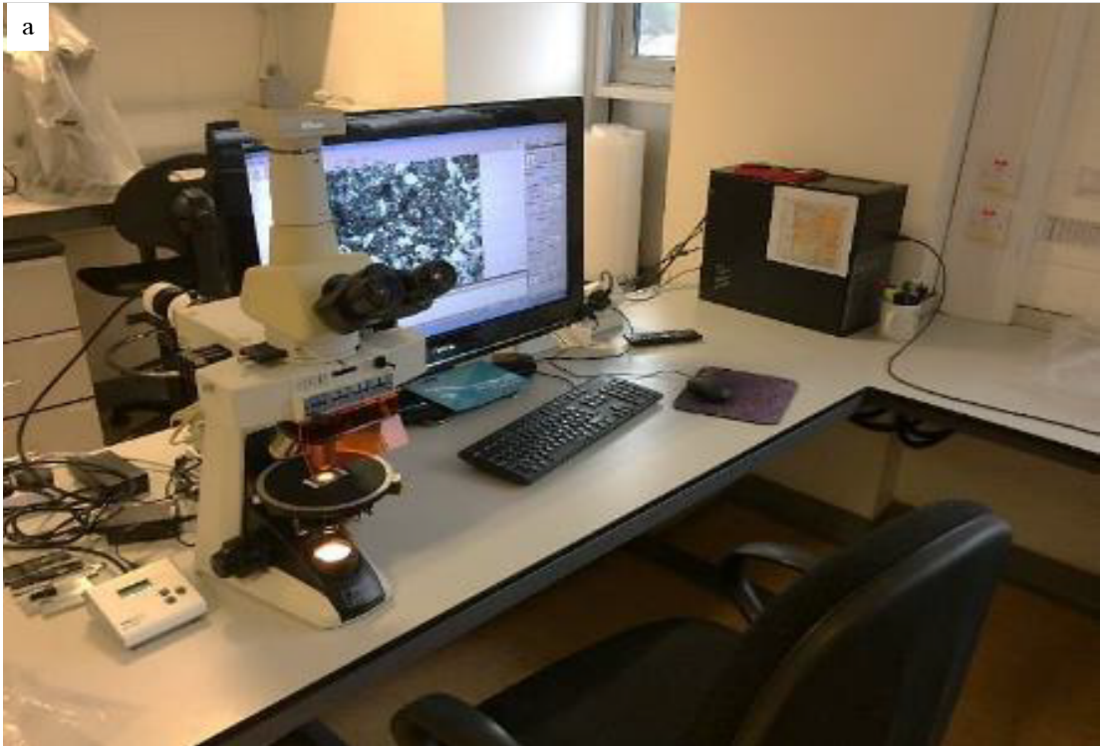
Figure 3.2: Transmitted Plane Polarised Light Microscope fitted with an incident UV light attachment used for microthermometric analysis of fluid inclusions at Geofluids Research Laboratory, National University of Ireland, Galway
